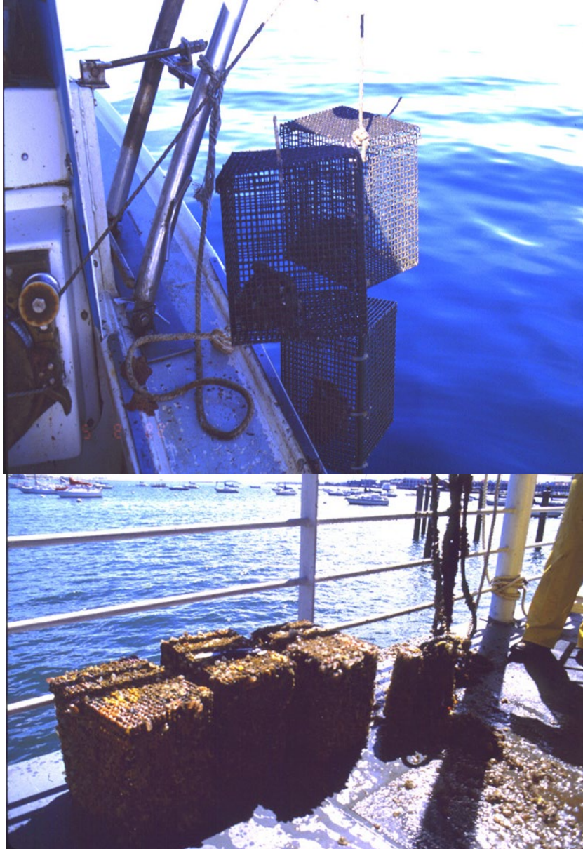
Figure 6-4. Pre- and post-deployment mussel cages. Mussels are collected from relatively pristine sites and deployed for periods of 40 and 60 days. Photo credit Battelle, Norwell, Massachusetts.
