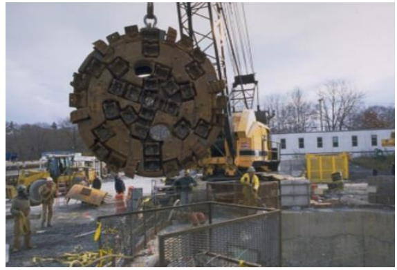
Example of tunnel boring machine cutting head
