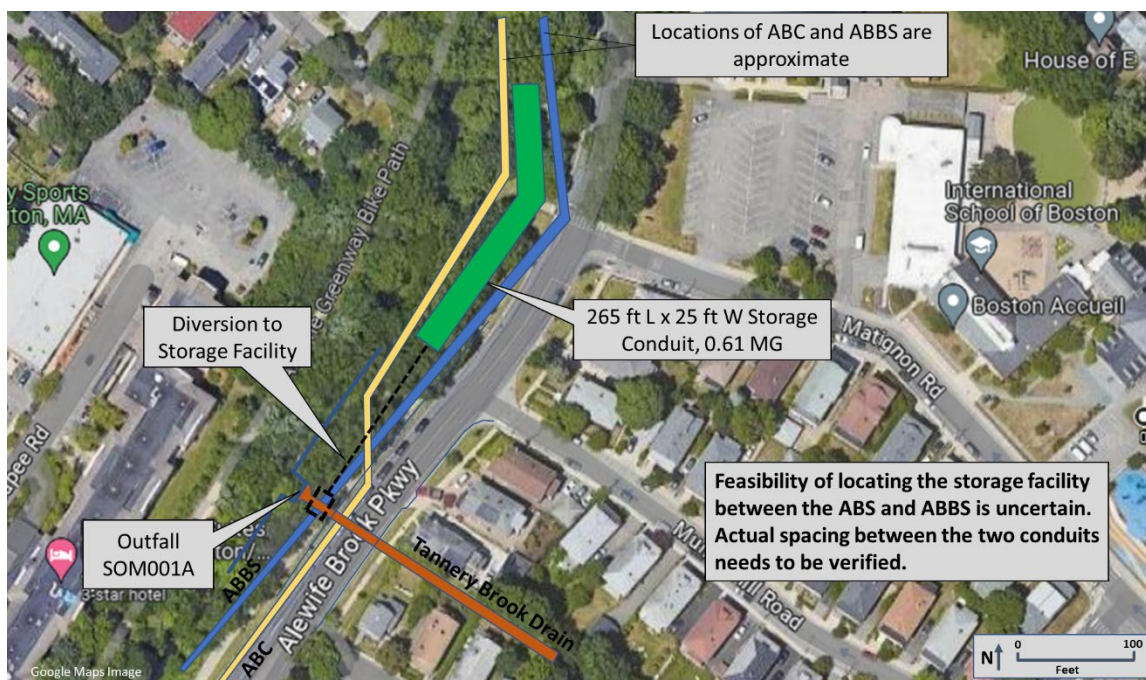
Figure 3-6. Box Conduit Storage Alternative for Outfall SOM001A
