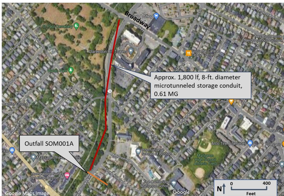
Figure 3-7. Microtunneled Storage Alternative for Outfall SOM001A
