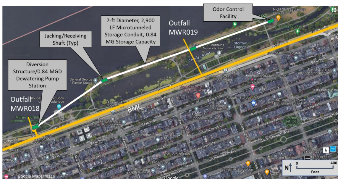
Figure 3-23. Microtunneled Conduit Storage Layout at Outfall MWR018
