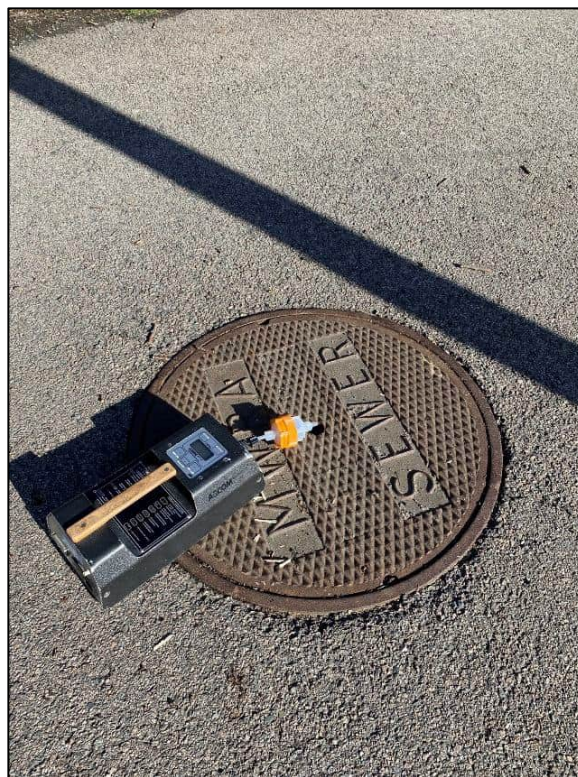
Figure 4-3. Handheld H 2 S Meter Sample Taken at ABC & ABBS Interceptor Connection #1 (Sta. 63+63) on 3/19/25 Along the Alewife Brook Parkway
