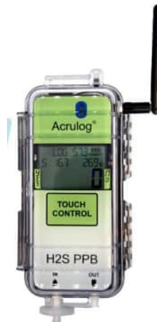
Figure 6-2. Example of Continuous Odor Monitoring Device (Acrulog)
