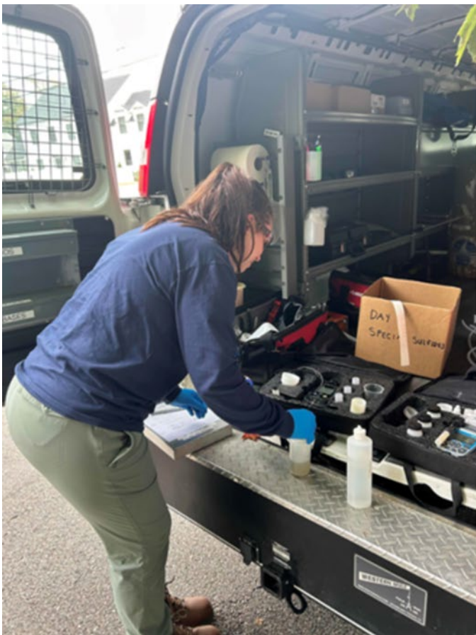
TRAC staff collecting and testing wastewater samples to monitor the collection system
