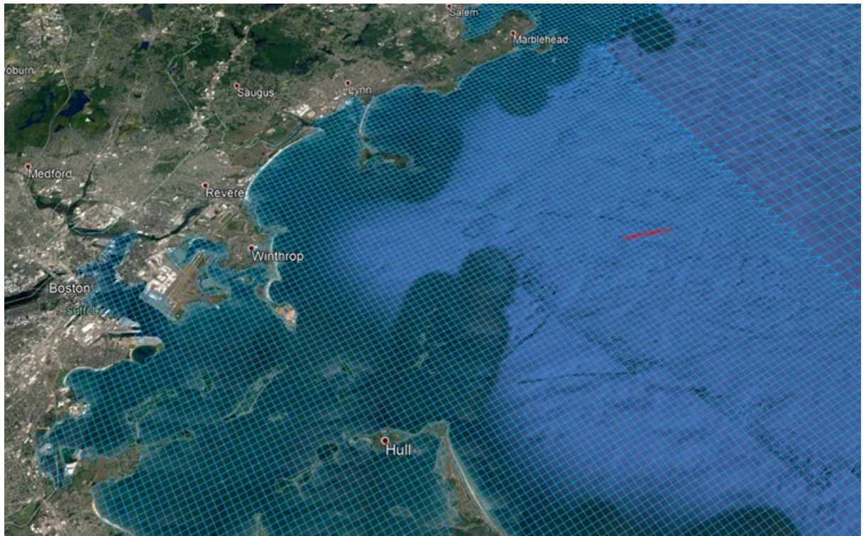
Figure A.4-1 Effluent diffuser array (red) and model grid (blue) in Boston area. The total MWRA-outfall discharge is evenly distributed over the 55 risers. The model grid has a resolution of 250m in the area of the outfall. The exact location of the risers and their bathymetric depths are given in Appendix A3.
