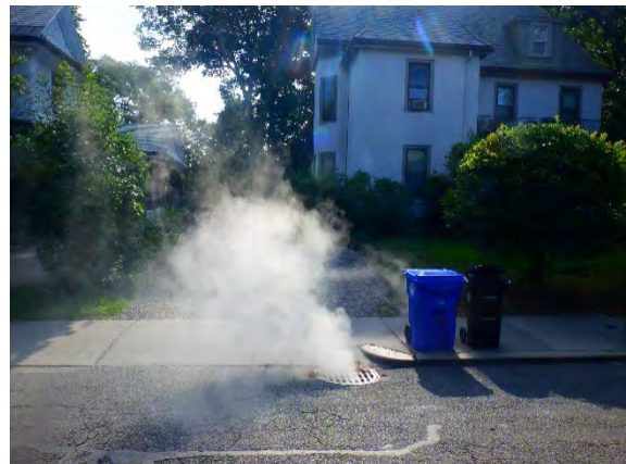
Identifying Inflow Sources by Smoke Testing
