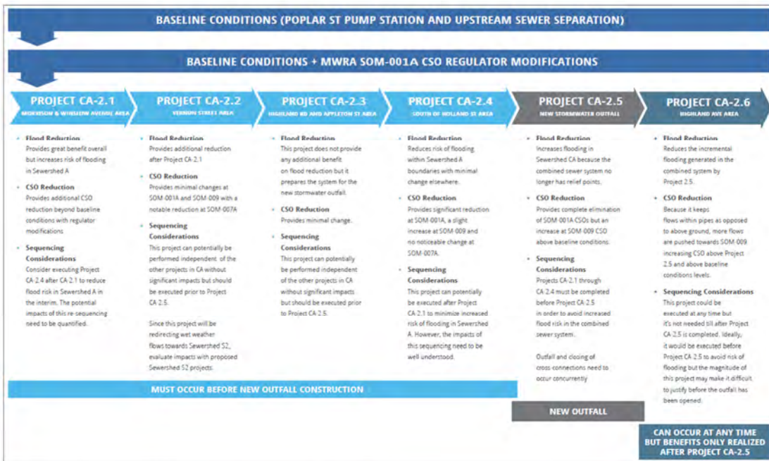
Figure 52. Recommended Project Sequencing with Flood Risk and CSO Considerations for Sewershed CA, Alternative 2 Projects
