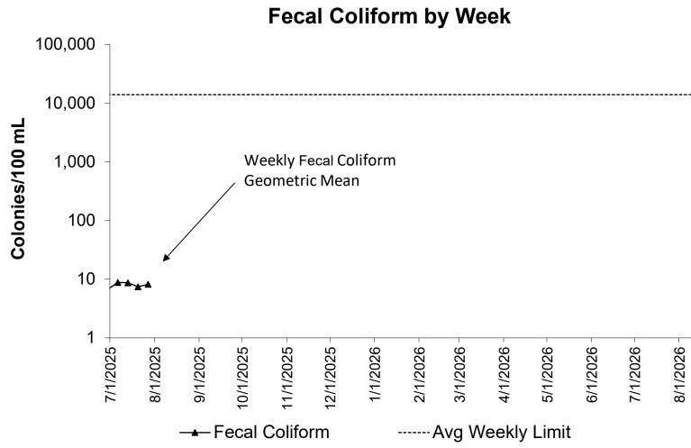
In July, all permit conditions for Fecal Coliform were met. Fecal Coliform is an indicator for the possible presence of pathogens. The levels of these bacteria after disinfection show how effectively the plant is inactivating many forms of disease-causing microorganisms.
