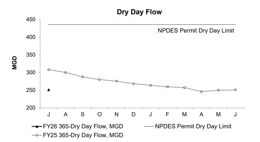
July's Dry Day Flow is the average of all dry weather influent flows over the previous 365 days from 8/1/2024 to 7/31/2025. The Dry Day Flow for the month was 251.5 MGD, well below the permit limit of 436 MGD.
