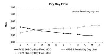
May's Dry Day Flow is the average of all dry weather influent flows over the previous 365 days from 6/1/2024 to 5/31/2025. The Dry Day Flow for the month was 249.9 MGD, well below the permit limit of 436 MGD.
