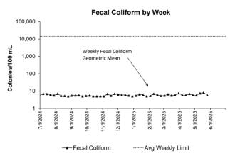
In May, all permit conditions for Fecal Coliform were met. Fecal Coliform is an indicator for the possible presence of pathogens. The levels of these bacteria after disinfection show how effectively the plant is inactivating many forms of disease-causing microorganisms.
