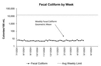
In April, all permit conditions for Fecal Coliform were met. Fecal Coliform is an indicator for the possible presence of pathogens. The levels of these bacteria after disinfection show how effectively the plant is inactivating many forms of disease-causing microorganisms.
