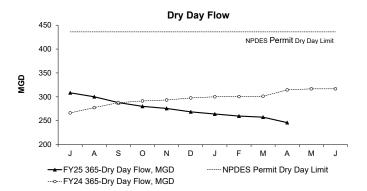
April's Dry Day Flow is the average of all dry weather influent flows over the previous 365 days from 5/1/2024 to 4/30/2025. The Dry Day Flow for the month was 246.0 MGD, well below the permit limit of 436 MGD.
