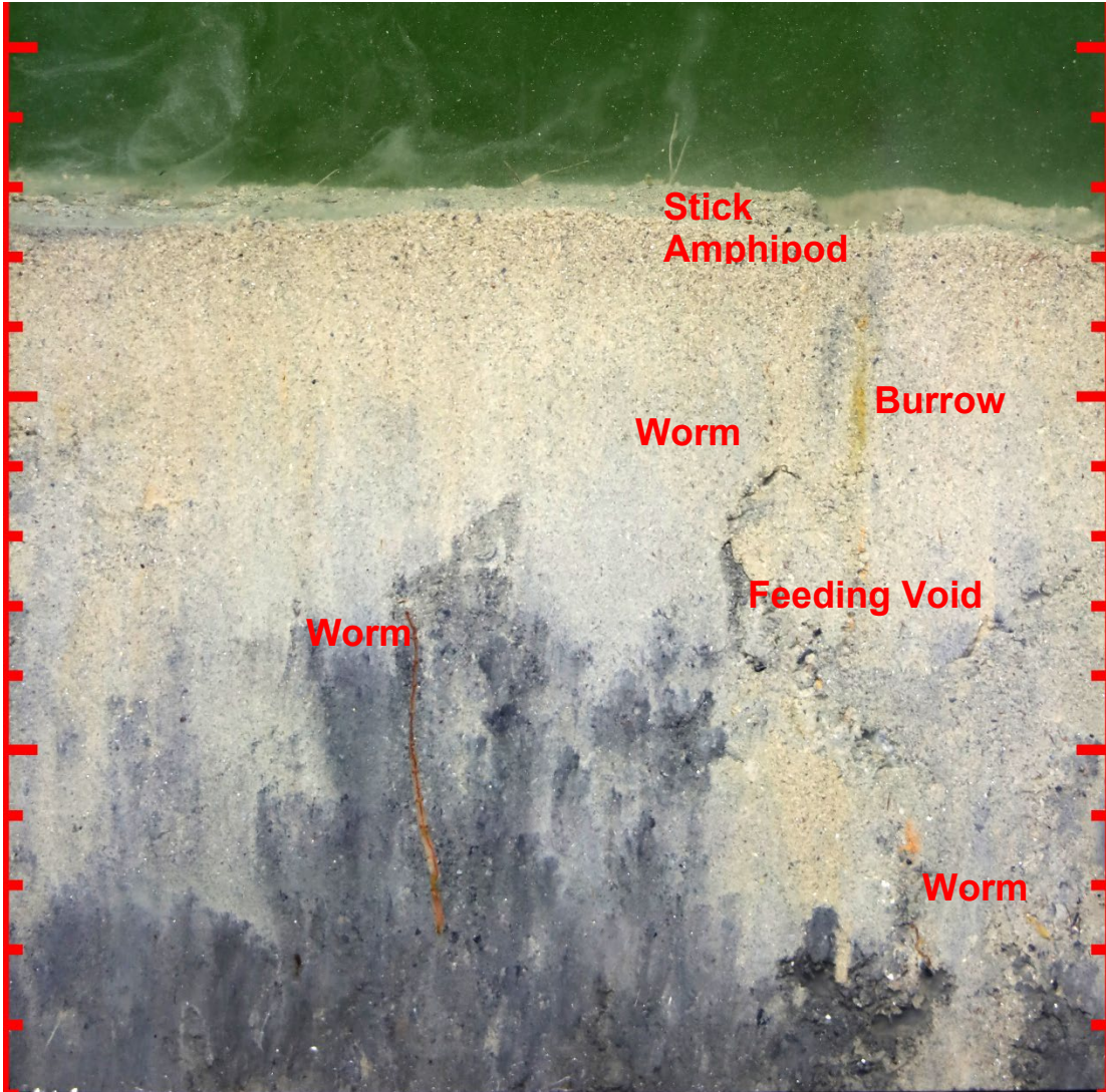
Figure 4-10. Example of a sediment-profile image taken in 2024 south of Deer Island and the north channel into the harbor. The change from light to dark color shows the transition from oxygenated to unoxidized sediment; this transition zone has deepened in response to improved conditions. Presence of organisms and feeding structures indicate a healthy environment. Scales at the sides of the image are in centimeters. Photo credit RJ Diaz and Daughters, Ware Neck, Virginia.
