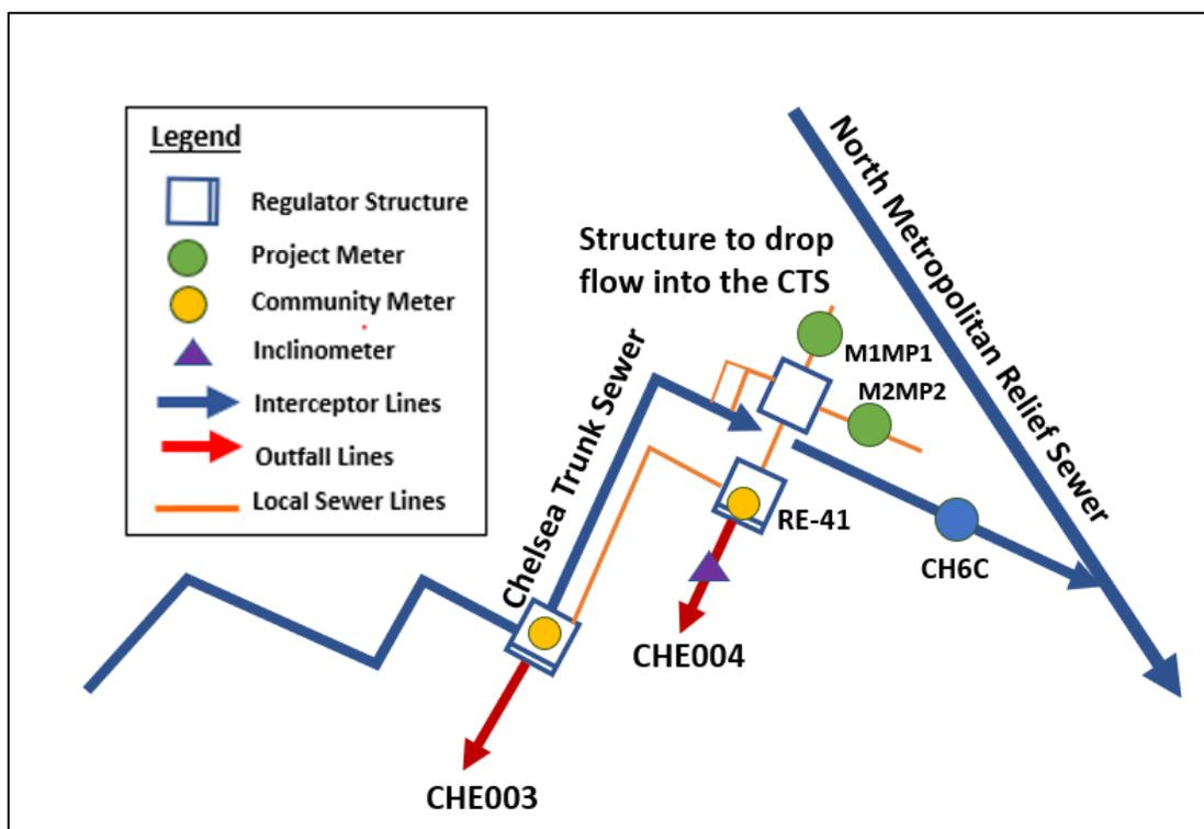
**Figure 2-7. Schematic of CHE004 Model Configuration**
