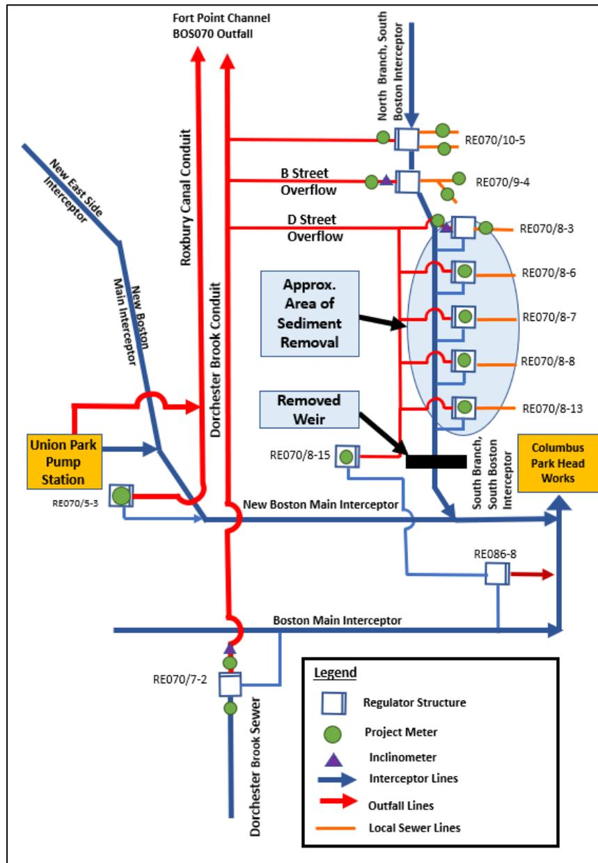
**Figure 2-5. Schematic of South Boston Interceptor System, Showing Location of Removed Maintenance Weir and Approximate Location of Sediment Removal**
