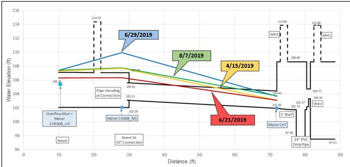
**Figure 2-9. Cross Section View of Regulator RE-081 and Connection to Interceptor**
