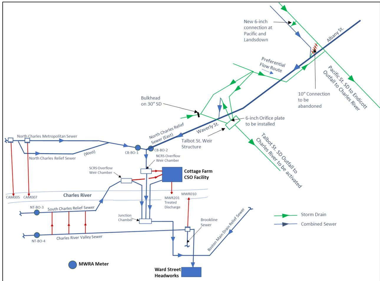
**Figure 2-4. Schematic of Cambridge Partial Sewer Separation Work**
