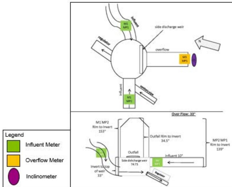
Figure 5-1. Example Regulator Schematic for RE009-2
