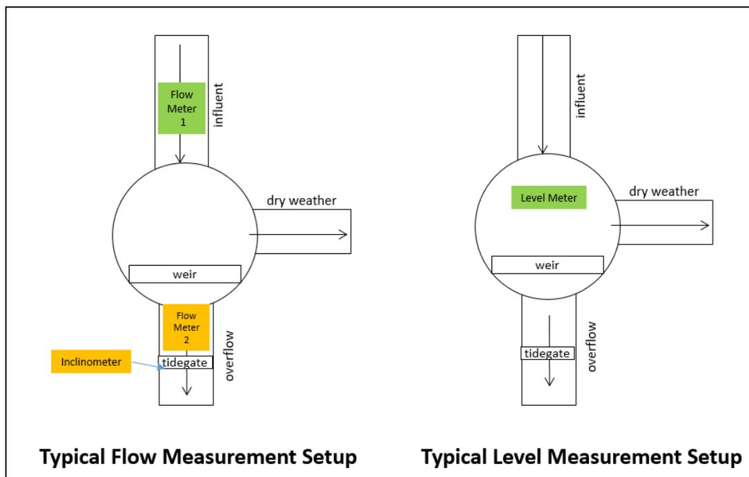
Figure 3-1. Example Meter Setup at a Generic Regulator Structure (Plan View Shown)
