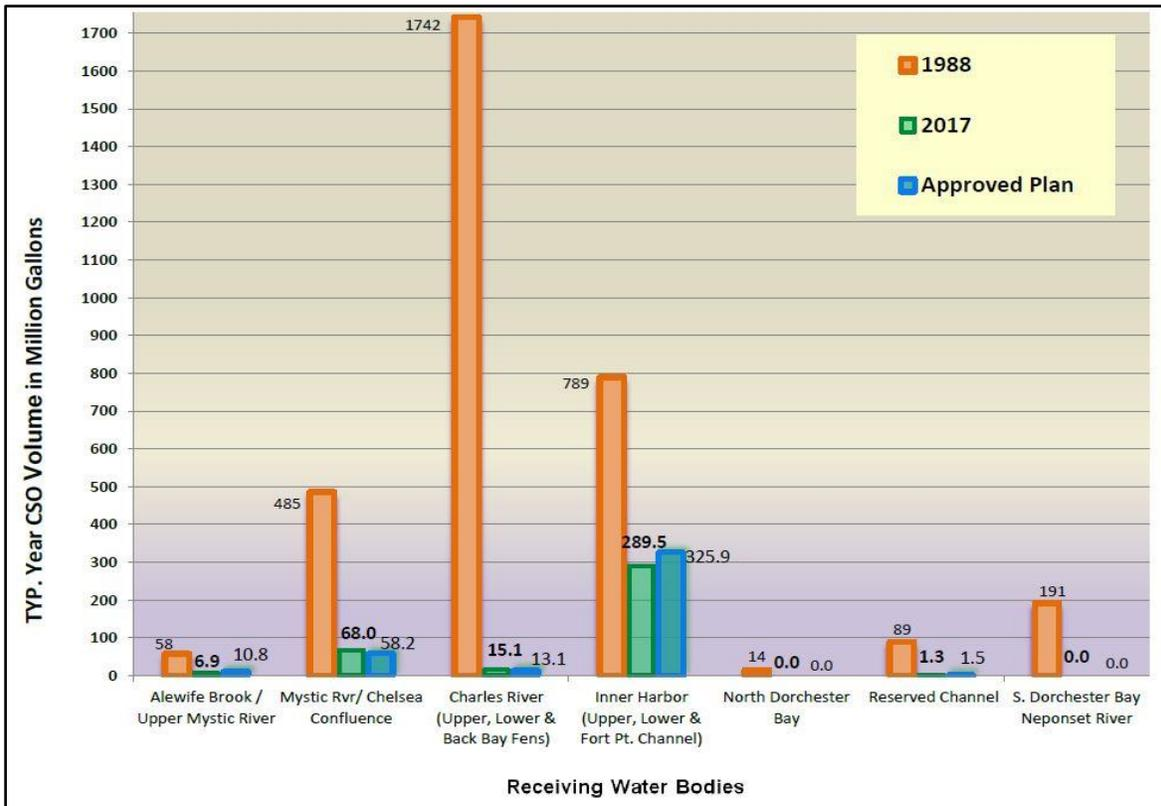
Figure 1-4. Region-wide CSO Discharge Volume Reduction by Receiving Water\*
