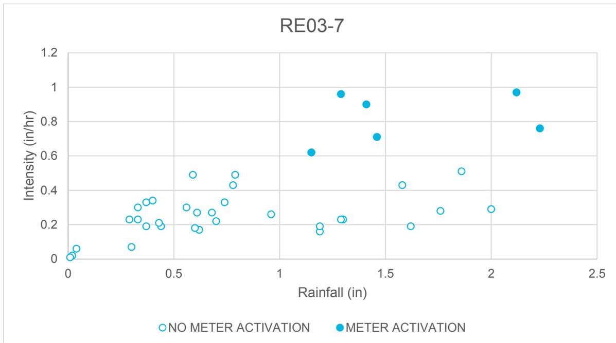
**Figure 4-4: Meter Review Scattergraph for Regulator RE03-7**
