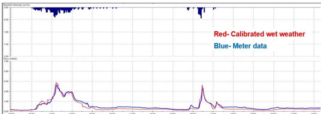
Figure 5-4. RE003-12 Influent Meter Calibration Plot
