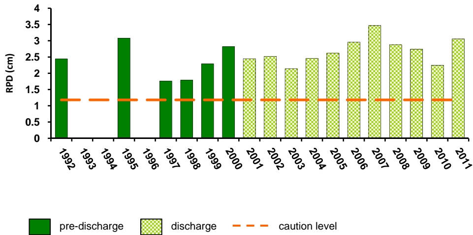
Figure 3 . Depth of the average redox potential discontinuity (RPD) in nearfield sediments as measured from sediment profile images, 1992-2011. RPDs in 2011 are among the deepest measured during discharge monitoring.
