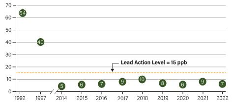
you drink. MWRA's water is lead-free when it leaves our reservoirs. Water mains are made mostly of iron, steel or concrete, and do not add lead to the water. Lead can enter your tap water from your service line (the line that connects your home to the water main) if it is made of lead, lead solder used in plumbing, or from some older brass faucets.
