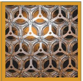
Ozone consists of three atoms of oxygen. It is created by applying an electrical current to pure oxygen in a specially designed chamber. Ozone provides better disinfection than chlorine alone, especially against *Cryptosporidium* and other hard to kill germs. It also reduces the amount of potentially harmful chlorine byproducts.
