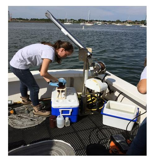
Grab samplers and sensors are used to take samples and measurements below the surface.
