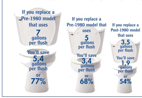
Whether you replace one toilet in a single bathroom or several hundred toilets in a large commercial or residential complex, you can expect to see significant savings. For example, replacing a typical 3.5 gallon toilet with a 1.6 gallon model will save a family of four 11,096 gallons per year. That's a 54% reduction in toilet water use. The more water the toilet you're replacing uses, the more you'll save.
