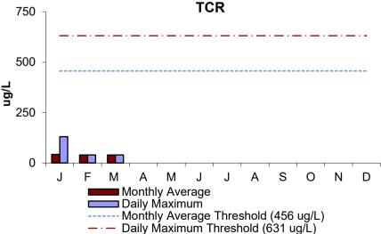
Total Chlorine Residual is the concentration of chlorine in the effluent as it leaves the treatment plant. Chlorine levels will drop off significantly as the effluent travels the length of the 9.5 mile outfall pipe. On this graph, we used the detection limit of 40 ug/L for values below detection.
