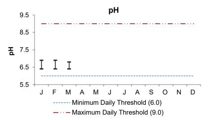
pH is a measure of alkalinity or acidity. The figure above plots the monthly range of pH measurements compared to permit limits. Fluctuations in effluent pH are unlikely to impact marine evironments, which have significant buffering capacity. Effluent pH tends to be at the lower end of the permit-required range due to the pure oxygen used in the activated sludge process. All pH measurements were within the threshold range for the quarter.
