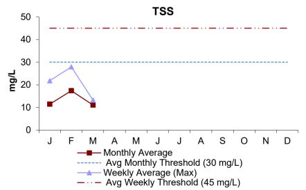
Total Suspended Solids is a measure of the amount of solids that remain suspended after treatment. The weekly and monthly concentrations for the quarter were below threshold values. The TSS percent removal range for the quarter was 79.5-87.4%
