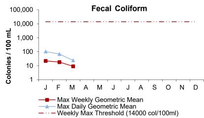
Fecal coliform is an indicator of the presence of pathogens. The levels of these bacteria after disinfection show how effectively the plant is inactivating disease-causing microorganisms. The Contingency Plan requires that the monthly geometric mean not exceed 14000 col/100mL. The monitoring results for the quarter were well below the threshold value.
