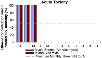
The acute toxicity test simulates the short-term toxic effects of pollutants in sewage effluent on marine animals. The test measures the concentration (percent) of effluent that kills half the test organisms within four days. The higher the concentration of effluent required, the less toxic the effluent. For permit compliance, the effluent concentration that causes mortality to mysid shrimp and inland silverside must be at least 50%. The threshold limits were met for the quarter.
