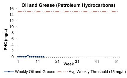
This graph shows levels of petroleum hydrocarbons in the DITP effluent. Samples were collected 5-6 times a month during the quarter. The Contingency Plan Threshold warning level is 15 mg/L weekly average. Since PHCs are lighter than water, they rise to the surface and are easily collected as scum from the primary and secondary clarifiers at DITP.
