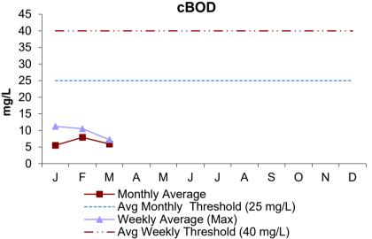
cBOD is a measure of the amount of dissolved oxygen required for the decomposition of organic materials in effluent. The weekly and monthly concentrations for the quarter were below threshold values. The 5-day cBOD percent removal range for the quarter was 90.4 -91.3
