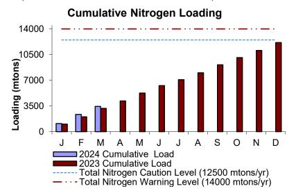
Total nitrogen is not regulated under the permit, but the Contingency Plan requires it to be closely monitored because of its potential effects on Massachusetts Bay. Total nitrogen includes total Kjeldahl nitrogen, nitrate, and nitrite.
