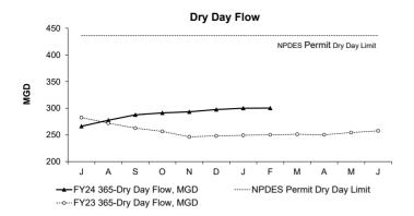
February's Dry Day Flow is the average of all dry weather influent flows over the previous 365 days from 3/1/2023 to 2/29/2024. The Dry Day Flow for the month was 300.4 MGD, well below the permit limit of 436 MGD.
