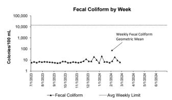
In February, all permit conditions for Fecal Coliform were met. Fecal Coliform is an indicator for the possible presence of pathogens. The levels of these bacteria after disinfection show how effectively the plant is inactivating many forms of disease-causing microorganisms.
