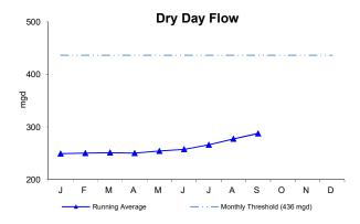
The dry day flow is calculated by averaging influent flow over the previous 365 days during dry weather. A dry day is defined as a day with < 0.09 inches of precipitation and no snow melt. In addition, the precipitation for the previous three days must be less than 0.3, 1.0, and 2.0 inches, respectively.
