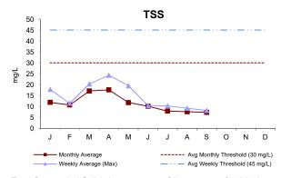
Total Suspended Solids is a measure of the amount of solids that remain suspended after treatment. The weekly and monthly concentrations for the quarter were below threshold values. The TSS percent removal range for the quarter was 91.5-92.2%
