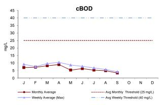
cBOD is a measure of the amount of dissolved oxygen required for the decomposition of organic materials in effluent. The weekly and monthly concentrations for the quarter were below threshold values. The 5-day cBOD percent removal range for the quarter was 94.3 -96.4%.
