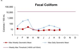
Fecal coliform is an indicator of the presence of pathogens. The levels of these bacteria after disinfection show how effectively the plant is inactivating disease-causing microorganisms. The Contingency Plan requires that the monthly geometric mean not exceed 14000 col/100mL. The monitoring results for the quarter were well below the threshold value.
