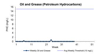
This graph shows levels of petroleum hydrocarbons in the DITP effluent. Samples were collected 5-6 times a month during the quarter. The Contingency Plan Threshold warning level is 15 mg/L weekly average. Since PHCs are lighter than water, they rise to the surface and are easily collected as scum from the primary and secondary clarifiers at DITP.
