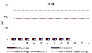
Total Chlorine Residual is the concentration of chlorine in the effluent as it leaves the treatment plant. Chlorine levels will drop off significantly as the effluent travels the length of the 9.5 mile outfall pipe. On this graph, we used the detection limit of 40 ug/L for values below detection.
