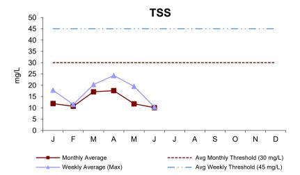
Total Suspended Solids is a measure of the amount of solids that remain suspended after treatment. The weekly and monthly concentrations for the quarter were below threshold values. The TSS percent removal range for the quarter was 80.5-89.3%
