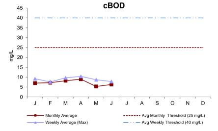
cBOD is a measure of the amount of dissolved oxygen required for the decomposition of organic materials in effluent. The weekly and monthly concentrations for the quarter were below threshold values. The 5-day cBOD percent removal range for the quarter was 90.2 -94,4%.
