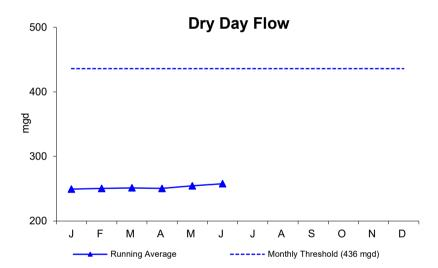
The dry day flow is calculated by averaging influent flow over the previous 365 days during dry weather. A dry day is defined as a day with < 0.09 inches of precipitation and no snow melt. In addition, the precipitation for the previous three days must be less than 0.3, 1.0, and 2.0 inches, respectively.
