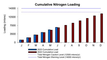
Total nitrogen is not regulated under the permit, but the Contingency Plan requires it to be closely monitored because of its potential effects on Massachusetts Bay. Total nitrogen includes total Kjeldahl nitrogen, nitrate, and nitrite.
