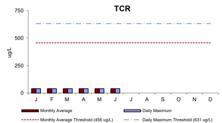
Total Chlorine Residual is the concentration of chlorine in the effluent as it leaves the treatment plant. Chlorine levels will drop off significantly as the effluent travels the length of the 9.5 mile outfall pipe. On this graph, we used the detection limit of 40 ug/L for values below detection.
