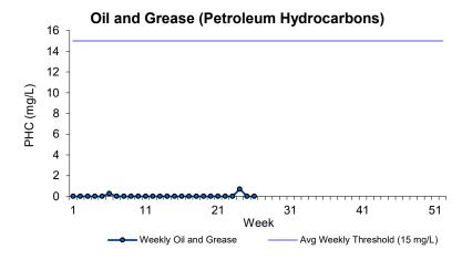
This graph shows levels of petroleum hydrocarbons in the DITP effluent. Samples were collected 5-6 times a month during the quarter. The Contingency Plan Threshold warning level is 15 mg/L weekly average. Since PHCs are lighter than water, they rise to the surface and are easily collected as scum from the primary and secondary clarifiers at DITP.
