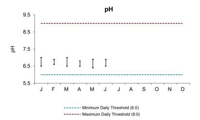
pH is a measure of alkalinity or acidity. The figure above plots the monthly range of pH measurements compared to permit limits. Fluctuations in effluent pH are unlikely to impact marine evironments, which have significant buffering capacity. Effluent pH tends to be at the lower end of the permit-required range due to the pure oxygen used in the activated sludge process. All pH measurements were within the threshold range for the quarter.
