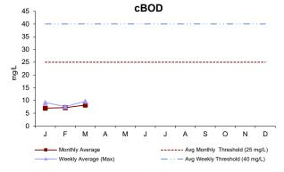
cBOD is a measure of the amount of dissolved oxygen required for the decomposition of organic materials in effluent. The weekly and monthly concentrations for the quarter were below threshold values. The 5-day cBOD percent removal range for the quarter was 90.2 - 93.3%.
