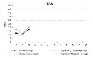
Total Suspended Solids is a measure of the amount of solids that remain suspended after treatment. The weekly and monthly concentrations for the quarter were below threshold values. The TSS percent removal range for the quarter was 87.6 - 94.3%
