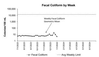
In December, all permit conditions for Fecal Coliform were met. Fecal Coliform is an indicator for the possible presence of pathogens. The levels of these bacteria after disinfection show how effectively the plant is inactivating many forms of disease-causing microorganisms.
