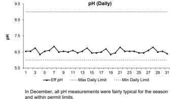
pH is a measure of the acidity or basicity of the effluent. Small fluctuations in pH do not have an adverse effect on marine environments. Because pure oxygen is used in the activated sludge reactors, the effluent pH tends to be at the lower range.
