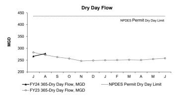
August's Dry Day Flow is the average of all dry weather influent flows over the previous 365 days from 9/1/2022 to 8/31/2023. The Dry Day Flow for the month was 277.5 MGD, well below the permit limit of 436 MGD.
