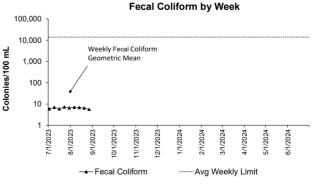
In August, all permit conditions for Fecal Coliform were met. Fecal Coliform is an indicator for the possible presence of pathogens. The levels of these bacteria after disinfection show how effectively the plant is inactivating many forms of disease-causing microorganisms.
