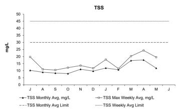
In May, both the weekly and monthly concentrations of TSS were below permit limits. The elevated TSS Monthly Avg and Max Weekly Avg in the effluent TSS is not uncommon during this time of the year due to the seasonal change in the wastewater temperature resulting in a shift in the biological activity of the secondary treatment microbes.
