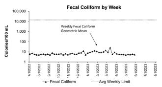
In May, all permit conditions for Fecal Coliform were met. Fecal Coliform is an indicator for the possible presence of pathogens. The levels of these bacteria after disinfection show how effectively the plant is inactivating many forms of disease-causing microorganisms.
