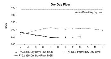
March's Dry Day Flow is the average of all dry weather influent flows over the previous 365 days from 4/1/2022 to 3/31/2023. The Dry Day Flow for the month was 251.3 MGD, well below the permit limit of 436 MGD. The Dry Day Flow had trended down through November 2022 due to much lower-than-expected plant flows from April 2022 through November 2022 due to the regional drought. Since then, plant flows have been at more typical levels.
