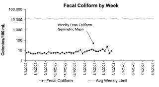
In March, all permit conditions for Fecal Coliform were met. Fecal Coliform is an indicator for the possible presence of pathogens. The levels of these bacteria after disinfection show how effectively the plant is inactivating many forms of disease-causing microorganisms
