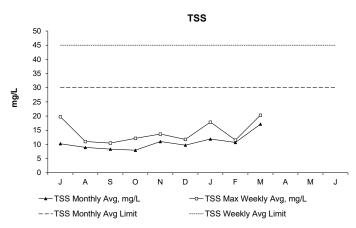
In March, both the weekly and monthly concentrations of TSS were below permit limits. The slightly elevated TSS Monthly Avg and Max Weekly Avg in March were due to the impacts of several significant rain/snow melt events, including a multi-day storm that triggered a continuous 45.33 hours of secondary blending, which resulted in periods of sustained high plant flows and a decrease in removal efficiencies as a result.
