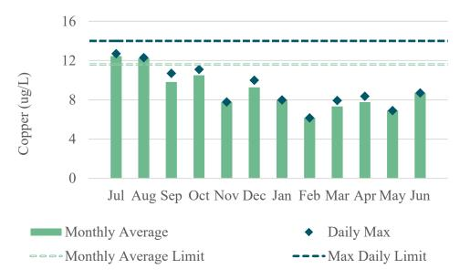
Figure 19. Effluent Copper Monthly Average and Daily Maximum Concentrations, FY23
