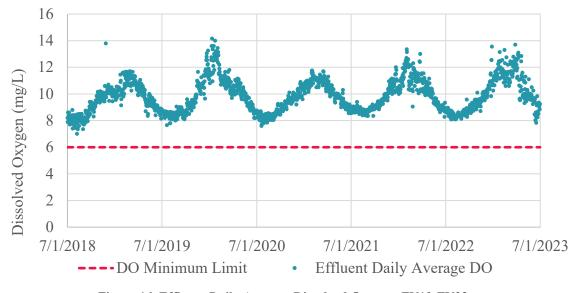
Figure 16. Effluent Daily Average Dissolved Oxygen, FY19-FY23
