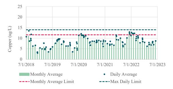
Figure 20. Effluent Copper Monthly Average and Daily Maximum Concentrations, FY19-FY23
