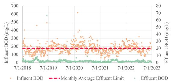
Figure 8. Influent and Effluent BOD Concentration Trends, FY19-FY23
