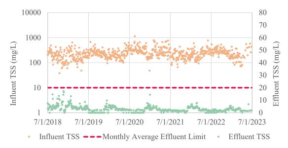
Figure 12. Influent and Effluent TSS Concentration Trends, FY19-FY23
