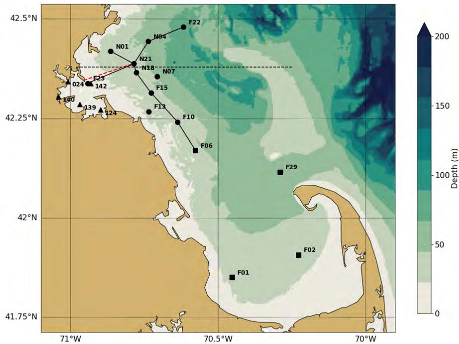
Figure 2-4 Location of MWRA monitoring locations (circles=Northern stations, squares=Southern stations, triangles=Harbor stations). The red dashed line indicates the tunnel between the DITP and the outfall diffusers. The black lines are the West-East and North-South transects used for model-observation comparisons of water quality constituents. The horizontal black dashed line represents the transect through the DITP outfall on which model results are presented in later figures.
