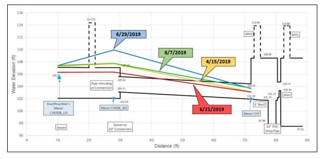
Figure 2-9. Cross Section View of Regulator RE-081 and Connection to Interceptor
