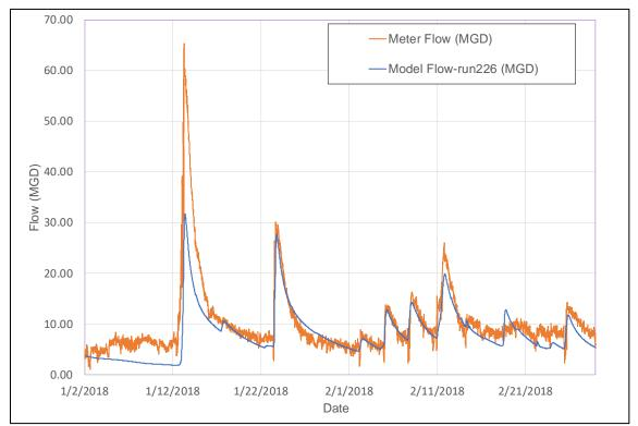
Figure 3-7. Measured and Calculated Flows at the Alewife Brook River Gauge for Jan-Feb, 2018
