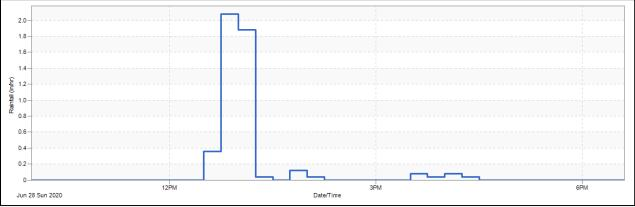
Figure 5-2. Hyetograph from the Ward Street Headworks Gauge for June 28, 2020
