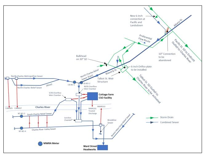
Figure 2-4. Schematic of Cambridge Partial Sewer Separation Work
