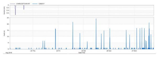
Figure 3-3. Example of Meter with Likely Incorrect Depth Measurements
