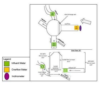
Figure 5-1. Example Regulator Schematic for RE009-2
