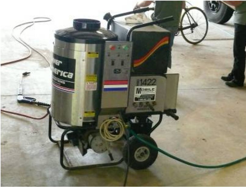
Photo: 6 Pressure washer used to steam clean and flush boat
