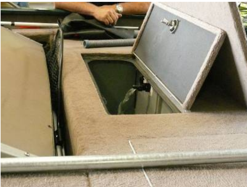
Photo: 11 Flushing live well supply lines
