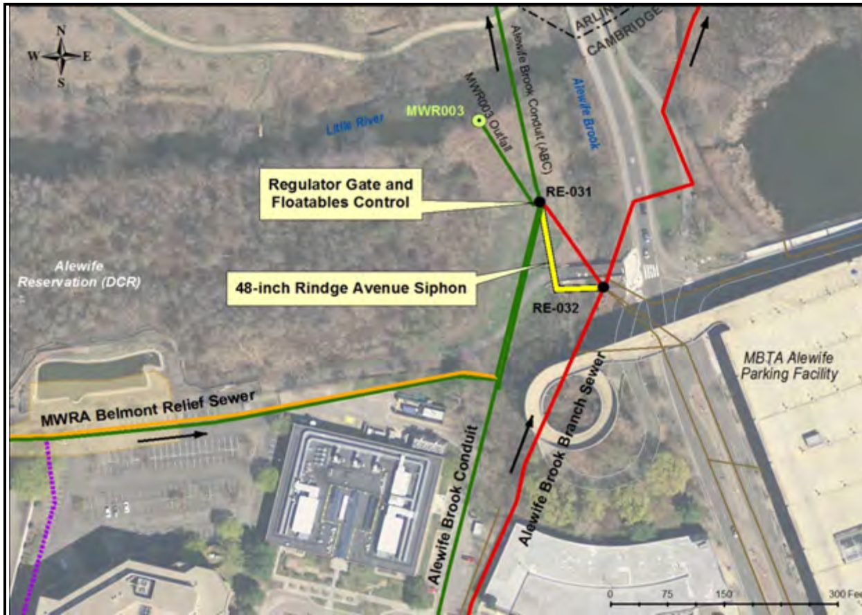
Figure 5: Control Gate and Floatables Control at Outfall MWR003 and MWRA Rindge Ave. Siphon Relief
