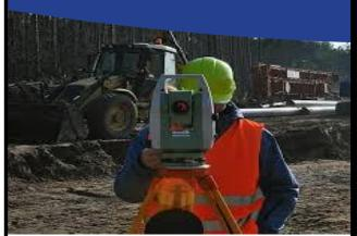
WHAT IS A FIELD SURVEY? Field survey is a method of locating surface features and ground elevations within the Program Study Area through the use of an instrument called a total station (pictured above).
