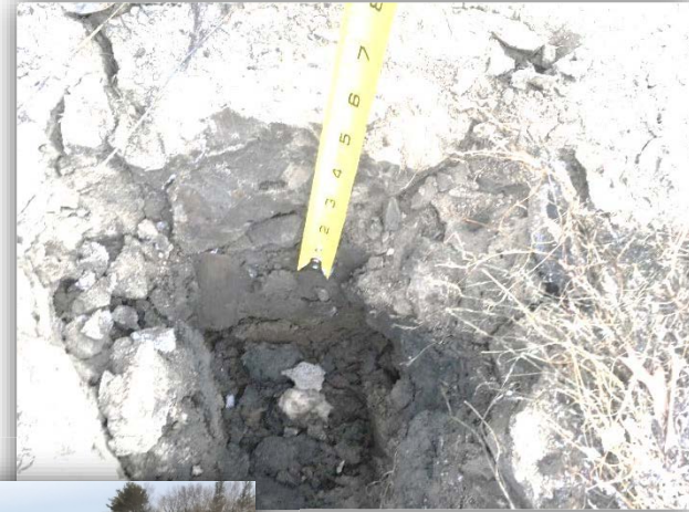
Small test hole to check freeze depth
