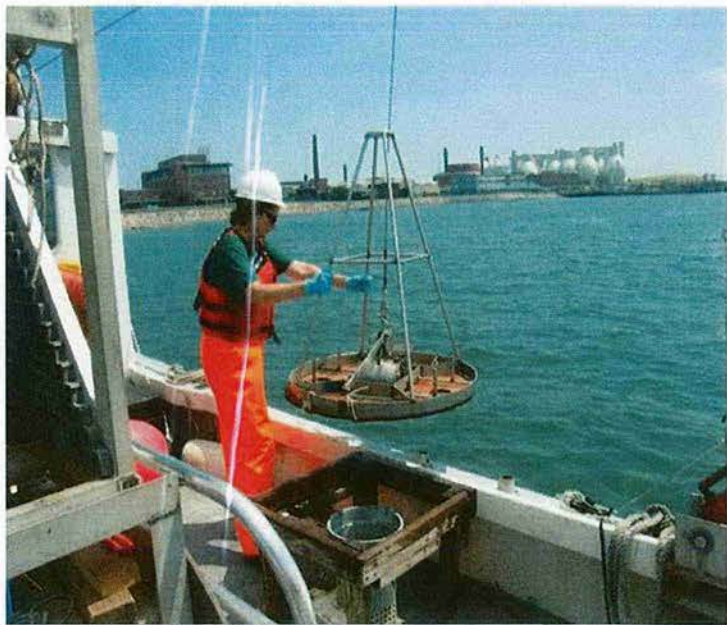
Figure 9. Collecting bottom sediment samples in Boston Harbor.
