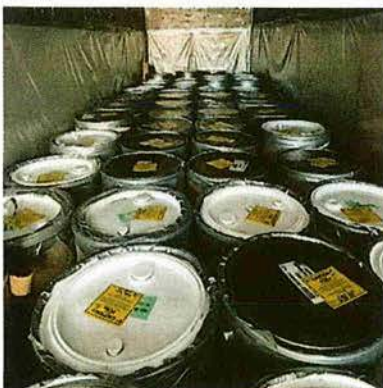
PCB waste containerized, labeled and stored for shipment to waste disposal site in Ohio
