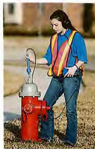
Leak Detection Technician "sounding" at a fire hydrant
