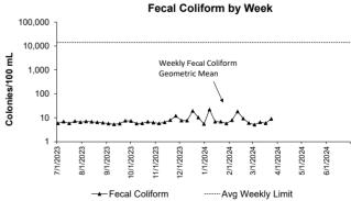
In March, all permit conditions for Fecal Coliform were met. Fecal Coliform is an indicator for the possible presence of pathogens. The levels of these bacteria after disinfection show how effectively the plant is inactivating many forms of disease-causing microorganisms.
