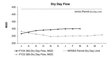
March's Dry Day Flow is the average of all dry weather influent flows over the previous 365 days from 4/1/2023 to 3/31/2024. The Dry Day Flow for the month was 301.2 MGD, well below the permit limit of 436 MGD.
