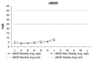
In January, both the weekly and monthly concentrations of cBOD were well below permit limits and within the expected ranges for this season. cBOD, or Carbonaceous Biochemical Oxygen Demand, is a measure of the amount of dissolved oxygen required for the decomposition of organic materials in the environment.
