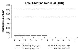
In January, both the maximum daily and monthly concentrations of TCR were below permit limits. TCR, or Total Chlorine Residual in the effluent, is a measure of the amount of chlorine that remains after the disinfection/dechlorination process. If the chlorine residual in the effluent is too high, it may threaten marine organisms.
