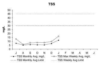
In January, both the weekly and monthly concentrations of TSS were below permit limits and within the expected ranges for this season. TSS typically trend slightly higher in the winter months due to slower settling as a result of the wastewater being denser, due to colder water temperatures, and also because plant flow in the winter are on average slightly higher. TSS, or Total Suspended Solids in the effluent, is a measure of the amount of solids that remain suspended after treatment.
