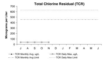
In November, both the maximum daily and monthly concentrations of TCR were below permit limits. TCR, or Total Chlorine Residual in the effluent, is a measure of the amount of chlorine that remains after the disinfection/dechlorination process. If the chlorine residual in the effluent is too high, it may threaten marine organisms.
