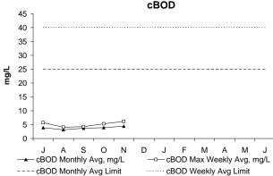
In November, both the weekly and monthly concentrations of cBOD were well below permit limits. cBOD, or Carbonaceous Biochemical Oxygen Demand, is a measure of the amount of dissolved oxygen required for the decomposition of organic materials in the environment.
