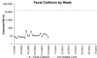
In November, all permit conditions for Fecal Coliform were met. Fecal Coliform is an indicator of the presence of pathogens. The levels of these bacteria after disinfection show how effectively the plant is inactivating many forms of disease-causing microorganisms.
