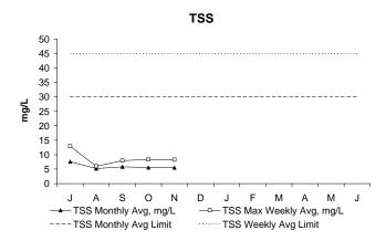
In November, both the weekly and monthly concentrations of TSS were below permit limits. TSS, or Total Suspended Solids in the effluent, is a measure of the amount of solids that remain suspended after treatment.
