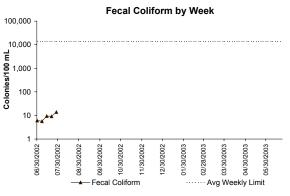
In July, all permit conditions were met. Fecal Coliform is an indicator of the presence of pathogens. The levels of these bacteria after disinfection show how effectively the plant is inactivating many forms of disease-causing microorganisms. There are 4 conditions in the permit that must be met: daily geomean; a weekly geomean; 10% of all samples; and three consecutive samples not to exceed 14,000 col/100mL.
