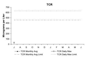
In July, both the maximum daily and monthly concentrations were below permit limits. Total Chlorine Residual in the effluent is a measure of the amount of chlorine that remains after the disinfection/dechlorination process. If the chlorine residual in the effluent is too high, it may threaten marine organisms.
