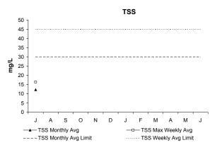
In July, both the weekly and monthly concentrations were below permit limits. Total Suspended Solids in the effluent is a measure of the amount of solids that remain suspended after treatment.
