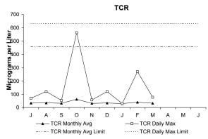
In March, both the maximum daily and monthly concentrations were below permit limits. Total Chlorine Residual in the effluent is a measure of the amount of chlorine that remains after the disinfection/dechlorination process. If the chlorine residual in the effluent is too high, it may threaten marine organisms.
