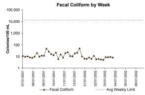
In March, all permit conditions were met. Fecal Coliform is an indicator of the presence of pathogens. The levels of these bacteria after disinfection show how effectively the plant is inactivating many forms of disease-causing microorganisms. There are 4 conditions in the permit that must be met: daily geomean; a weekly geomean; 10% of all samples; and three consecutive samples not to exceed 14,000 col/100mL.
