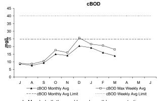
In March, both the weekly and monthly concentrations were below permit limits. Carbonaceous Biochemical Oxygen Demand is a measure of the amount of dissolved oxygen required for the decomposition of organic materials in the environment.
