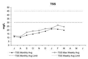
In March, both the weekly and monthly concentrations were below permit limits. Total Suspended Solids in the effluent is a measure of the amount of solids that remain suspended after treatment.
