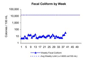
Fecal coliform is an indicator of the presence of pathogens. The levels of these bacteria after disinfection show how effectively the plant is inactivating many forms of disease-causing microorganisms. There are four conditions in the permit including daily geomean, a weekly geomean, 10% of all samples, and three consecutive samples not to exceed 14000 col/100mL. In March, all of these conditions were met.
