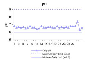
pH is a measure of the alkalinity or acidity of the effluent. Fluctuations in pH do not have an adverse effect on marine environments. Because of the pure oxygen used in the activated sludge reactor, the effluent pH tend to be at the lower pH range. In March, all pH measurements were within the permit limit range.
