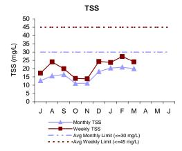
Total Suspended Solids in the effluent is a measure of the amount of solids that remain suspended after treatment. In March, both the weekly and monthly concentrations were below permit limits. The TSS removal rate was 85.2%.
