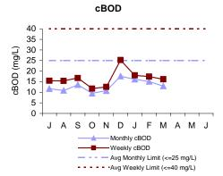
The cBOD is a measure of the amount of dissolved oxygen required for the decomposition of organic materials in effluent. In March, both the weekly and monthly concentrations were well below permit limits. The 5-day cBOD removal rate for March was 83.2%.
