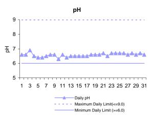
pH is a measure of the alkalinity or acidity of the effluent. Sudden change in pH does not have an adverse effect on marine environments. Because of the pure oxygen used in the activated sludge reactor, the effluent pH tend to be at the lower pH range. In January, all pH measurements were within the permit limit range.
