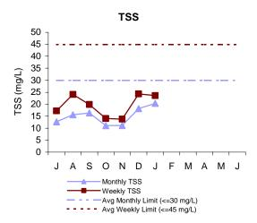
Total Suspended Solids in the effluent is a measure of the amount of solids that remain suspended after treatment. In January, both the weekly and monthly concentrations were below permit limits. The TSS removal rate was 90.3%.
