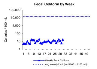
Fecal Coliform is an indicator of the presence of pathogens. The levels of these bacteria after disinfection show how effectively the plant is inactivating many forms of disease-causing microorganisms. There are four conditions in the permit including daily geomean, a weekly geomean, 10% of all samples, and three consecutive samples not to exceed 14000 col/100mL. In January, all of these conditions were met.
