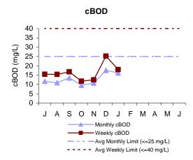
The cBOD is a measure of the amount of dissolved oxygen required for the decomposition of organic materials in the environment. In January, both the weekly and monthly concentrations were well below permit limits. The 5-day cBOD removal rate for January was 87.0%.
