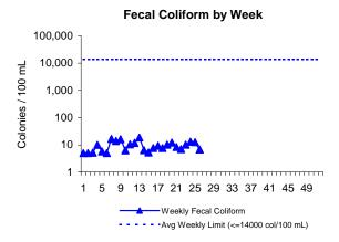
Fecal Coliform is an indicator of the presence of pathogens. The levels of these bacteria after disinfection show how effectively the plant is inactivating many forms of disease-causing microorganisms. There are four conditions in the permit including daily geomean, a weekly geomean, 10% of all samples, and three consecutive samples not to exceed 14000 col/100mL. In December, all of these conditions were met.
