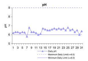
pH is a measure of the alkalinity or acidity of the effluent. Sudden change in pH does not have an adverse effect on marine environments. Because of the pure oxygen used in the activated sludge reactor, the effluent pH tend to be at the lower pH range. There was one low pH reading on December 7. All other measurements for the month of December were within the permit limit range.
