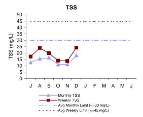
Total Suspended Solids in the effluent is a measure of the amount of solids that remain suspended after treatment. In December, both the weekly and monthly concentrations were below permit limits. The TSS removal rate was 88.9%.
