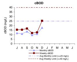
The cBOD is a measure of the amount of dissolved oxygen required for the decomposition of organic materials in the environment. In December, both the weekly and monthly concentrations were below permit limits. The 5-day cBOD removal rate for December was 83.4%.
