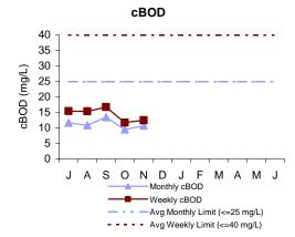
The cBOD is a measure of the amount of dissolved oxygen required for the decomposition of organic materials in the environment. In November, both the weekly and monthly concentrations were well below permit limits. The 5-day cBOD removal rate for November was 91%.
