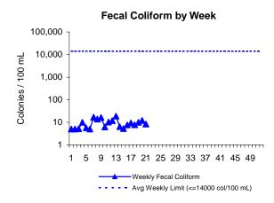
Fecal Coliform is an indicator of the presence of pathogens. The levels of these bacteria after disinfection show how effectively the plant is inactivating many forms of disease-causing microorganisms. There are four conditions in the permit including daily geomean, a weekly geomean, 10% of all samples, and three consecutive samples not to exceed 14000 col/100mL. In November, all of these conditions were met.
