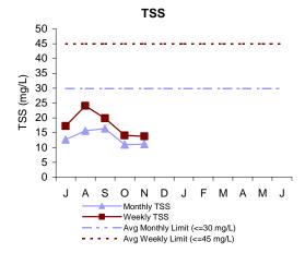
Total Suspended Solids in the effluent is a measure of the amount of solids that remain suspended after treatment. In November, both the weekly and monthly concentrations were well below permit limits. The TSS removal rate was 92%.
