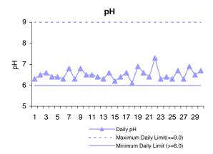
pH is a measure of the alkalinity or acidity of the effluent. Sudden change in pH does not have an adverse effect on marine environments. Because of the pure oxygen used in the activated sludge reactor, the effluent pH tend to be at the lower pH range. In November, all pH measurements were within the permit limit range.
