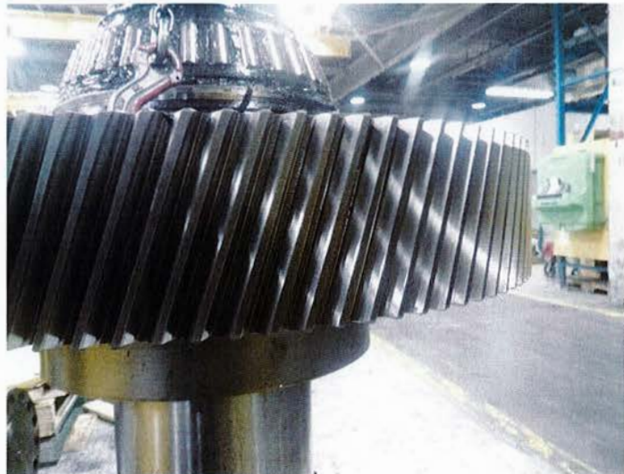
From Vendor's report, low-speed gear found with good wear pattern, suitable for reuse
