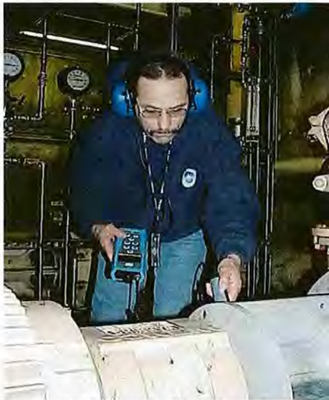
Acoustic Ultrasonic Checking of a Bearing
